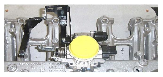
Install the new throttle body and gasket as shown.
