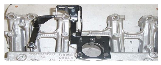
Remove your existing throttle body. Install the adapter and new three hole throttle body gasket using the three countersunk screws provided. Install the cable bracket support. Leave the mounting bolt loose at this time. Mount the throttle cable bracket on the extended section of the throttle body adapter and the bracket support. Tighten the 6mm cap screws. Tighten the support bracket mounting bolt at this time.
